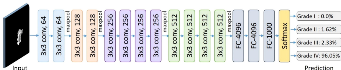
Fig. 3. Architecture of fine-tuned VGG-19 CNN model.
